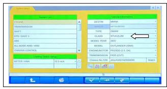
4. The System Select screen opens and populates with some basic information from the vehicle. Look at the label on the passenger side B pillar to identify the appropriate class. (See B pillar label below; class is labeled as "model"). If necessary, select the correct class from the drop-down list.
