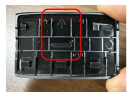
2. Remove the auxiliary key in the middle. Be careful not to drop or misplace the side fob buttons as they will become loose when you remove the key fob cover (buttons are in the red oval shape).
