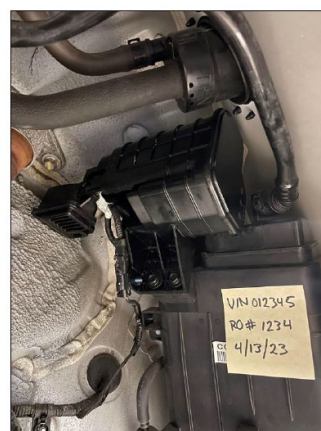
Acceptable STUI Photo of Canister Installed & Campaign Sticker Installed on Vehicle
