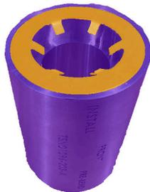
8. Install the front washer sleeve into the outer sleeve. Make sure that the side of the tool labeled "INSTALL" points toward the vehicle.
