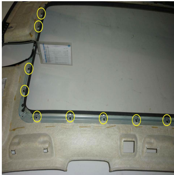
Figure 1. Location of the headliner to sunroof frame clips.
