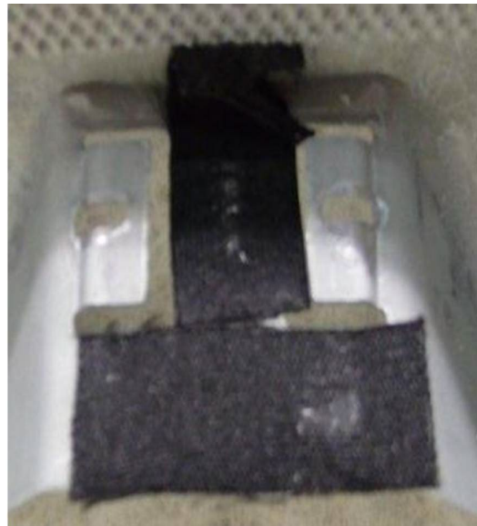
Figure 2. Location of the webbing adhesive tape application.
