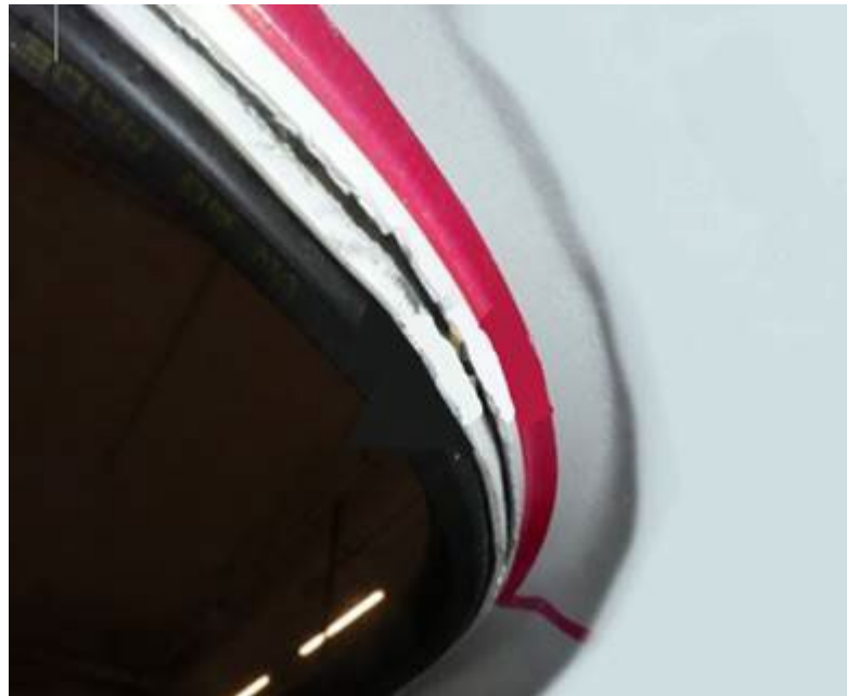
Figure 8. Create a gap of approximately 1mm.
