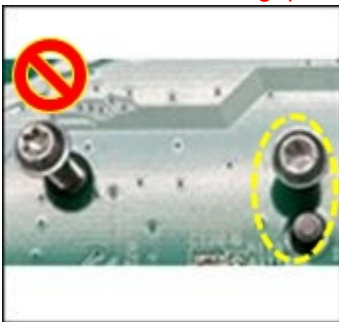
Locating pin and screw
