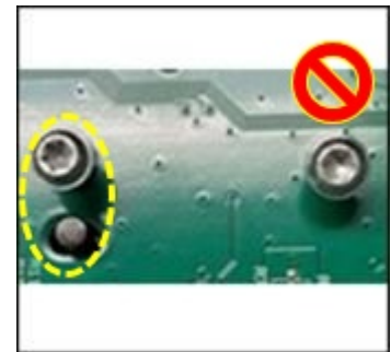
Locating pin and screw
