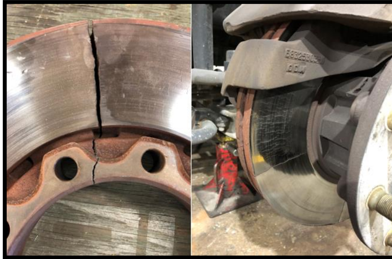
(Example of failed rotors)
