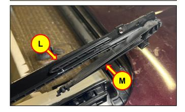
Install the locking tab of the new driving wedge (M) into the locking slide (O) of the sunroof mechanism.
