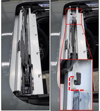
8. While lifting the rear of the carriage bar (L), separate the driving wedge (M) from the curve guides.
