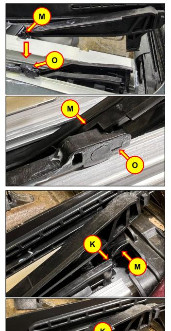
19. Lower the new driving wedge (M) and insert it in between both curve guides (K).
