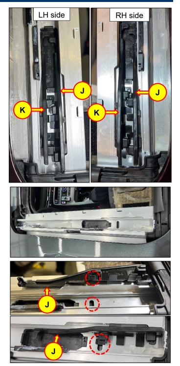
15. Install the new curve guide B (K) into the sunroof mechanism rail.
