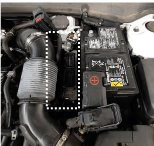
3. Remove two bolts securing Control Harness to Intake Manifold.
