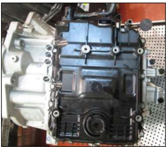
26. Remove the transaxle fill plug.
