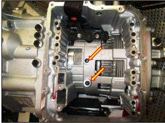
19. Align the manual shaft to the shift lever and install the valve body.
