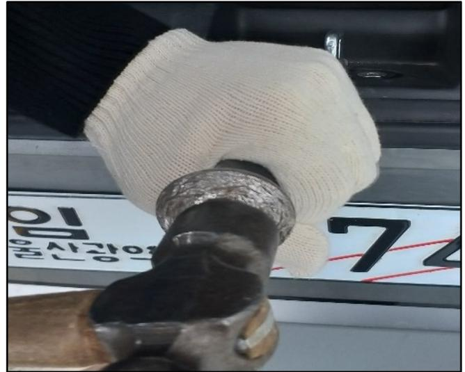
9. Tighten the screws (D) on the tailgate striker.
