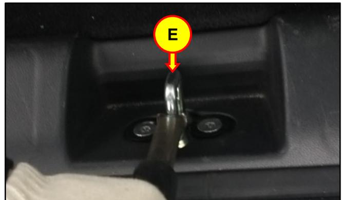
8. Hit the striking pry bar with a hammer 5 times using moderate force.
