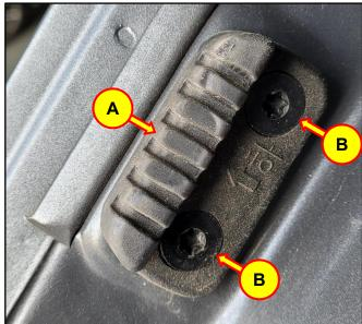
3. Install 3 washer pads on each screw on the backside of the side guide bumper.
