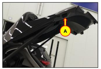
2. Remove the screws (B) and remove the side guide bumper (A).
