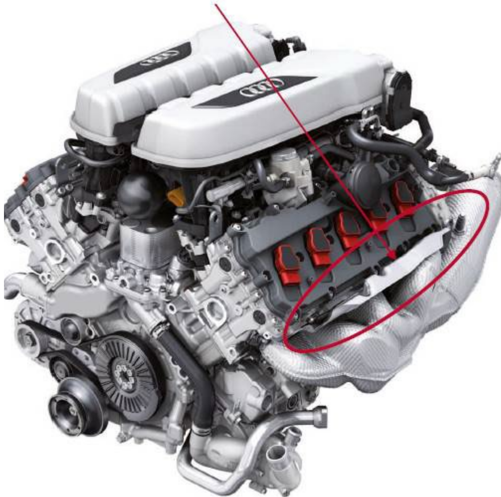
Figure 4: The manifold heat shield is circled in red.
