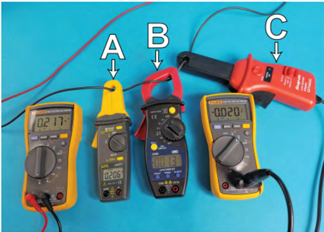
Figure 11-29 A) Stand alone low amperage induction clamp B) Stand alone high amperage inductive clamp C) DVOM dependent low amperage inductive clamp
