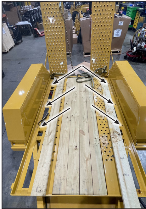
Figure 12 Holes Drilled in Frame
