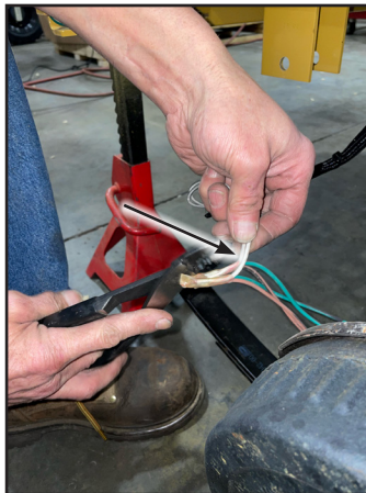
Figure 4 Cut White Wires
