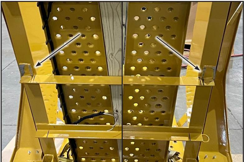
Figure 6 Hangers Cut Off
