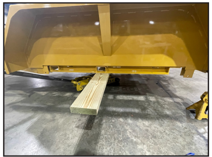
Figure 10 Subframe Lifted into Place
