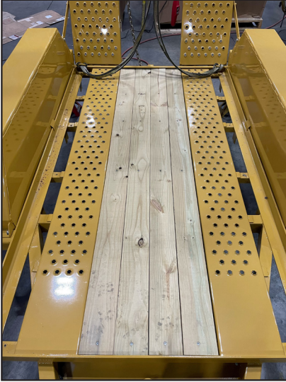
Figure 2 Outside Boards Removed
