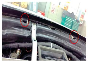
2. Apply a felt strip to both the bulkhead upper part and to the dashboard.
