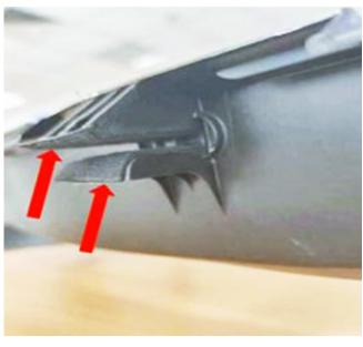
Location of both felt strips, on the upper and lower prongs of the dashboard retaining clips.
