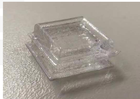
Figures 1: Overlapping and glued pads
