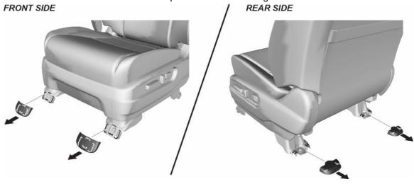
2. Remove the four seat mounting bolts. FRONT SIDE
