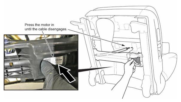
9. Disconnect the other end of the flex cable assembly from the seat rail gearbox side. Do not bend or kink the cable. NOTE: The cable may be tight in the gearbox. Use needle nose pliers to remove the cable.
