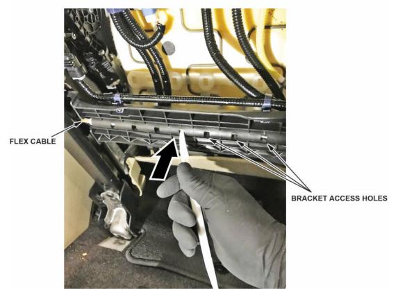
8. Disconnect the flex cable from the motor side first by gently pushing in on the motor at the cable end to disengage it from its mounting bracket. This will help when removing and replacing the flex cable assembly.
