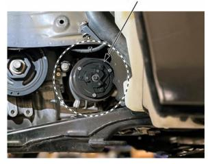
6. If no oil is noticed, leave the compressor on the vehicle. Remove the center hub bolt and hub/armature plate from the compressor. Then, inspect both for oil
