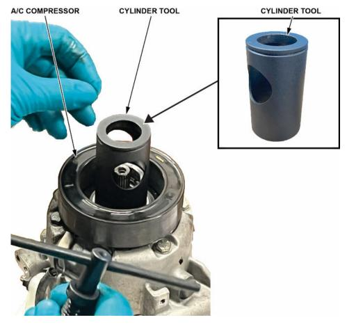
19. Insert the extractor tool, and make sure the **24 mm** nut is positioned towards the top.Look into the cylinder window to align the extractor tool onto the flange and press the handle fully down to grab the seal.
