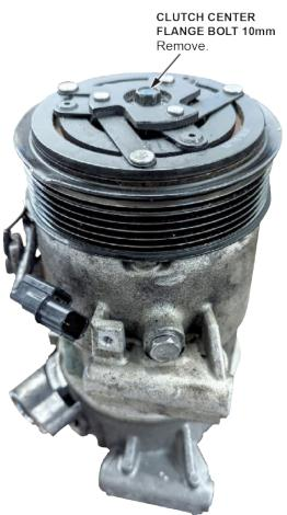
6. If the clutch has not been removed from a previous step, remove the clutch while being careful not to drop/lose any shims (usually 1–2).
