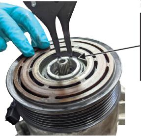
PULLEY OUTER C-RING Remove.
