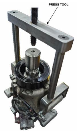
32. Tighten the press by rotating the handle clockwise until it reaches the adapter tool. Slowly and carefully continue to rotate the handle clockwise until the seal is pressed down roughly **10 mm** below the bore.
