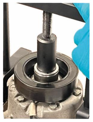
17. Release to remove the adapter and press.
