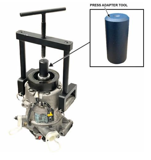
15. Add grease to the press adapter button and press threads.
