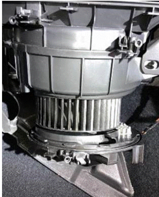
Figure 4. Fresh air blower V2 removal.
