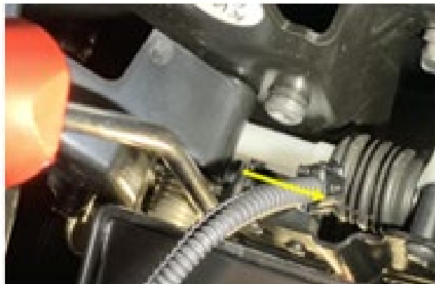
Figure 3. Slide only Bowden cable toward actuator.
