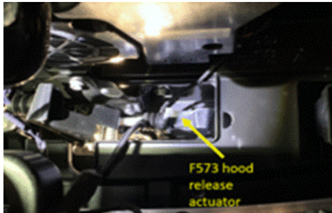
Figure 2. Hood latch release actuator location.
