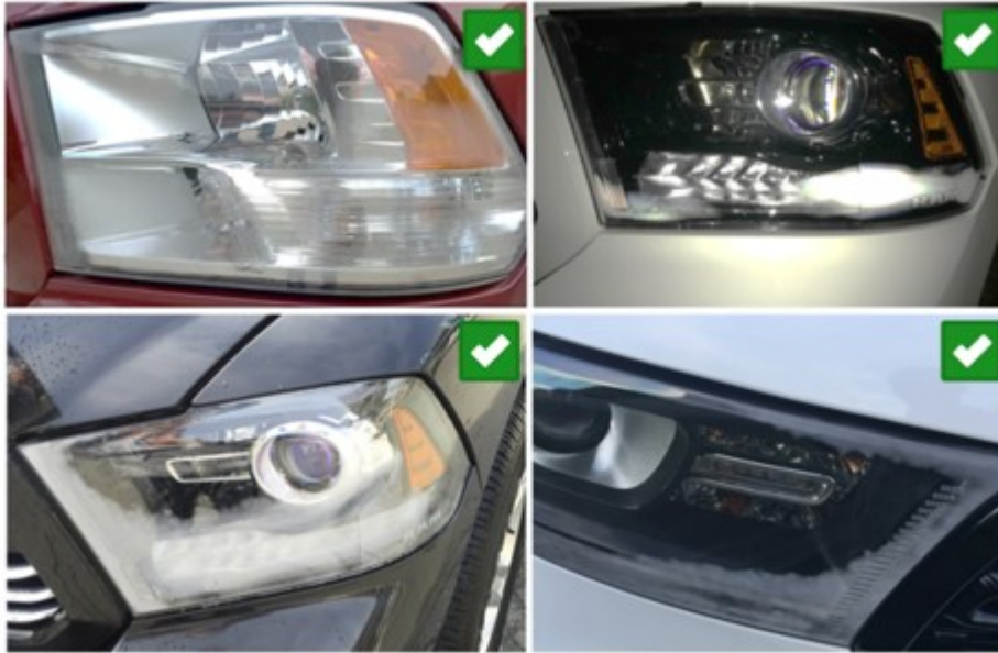
Fig. 2 Condensation/Fogging Begun To Clear
