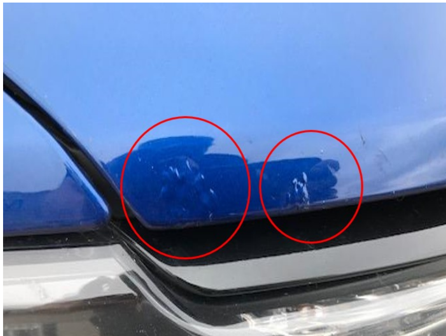
Fig. 3 Examples of Corrosion Along Leading Edges
