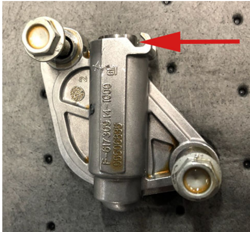
Photo below shows the timing tensioner removed from engine. Note the plunger is stuck in body of tensioner.
