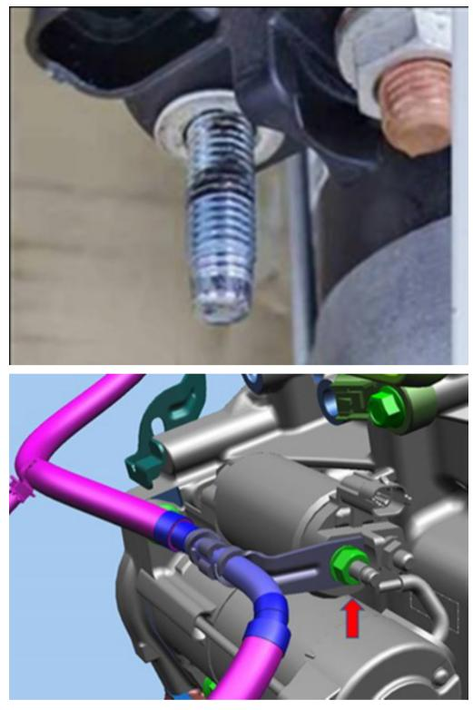
If it's oxidized as shown in the photos, you should replace the nut and clean the stud terminals and re-check starter function.
