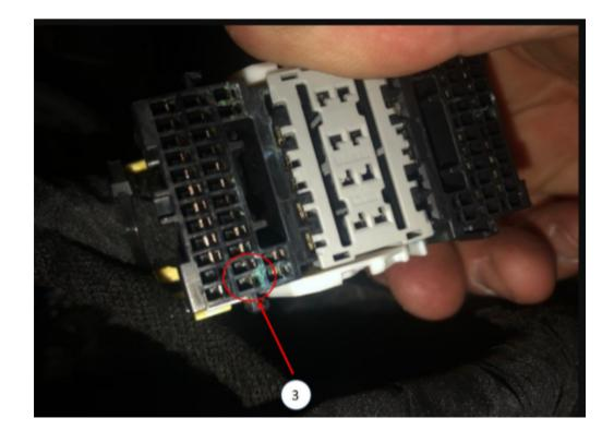
If any issues are found then follow SI Wiring and Connector repair instructions to correct the concern.
