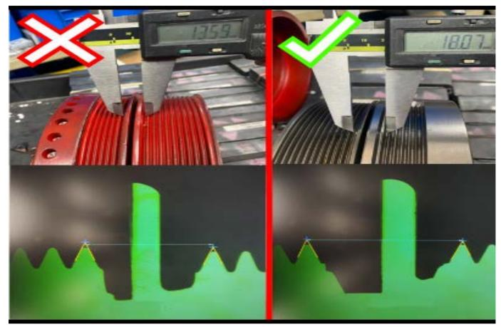
Good parts should measure 18mm +/- 1mm across ribs as shown in the graphic above.
