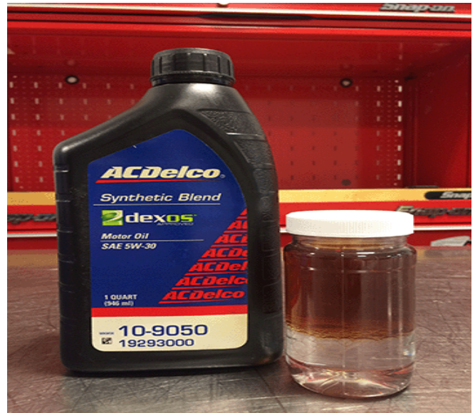
Diesel Exhaust Fluid (DEF) mixed with Engine Oil.
