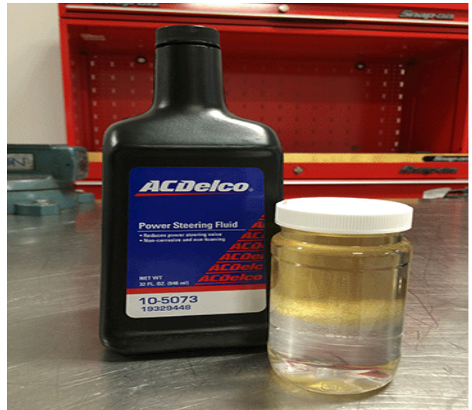
Diesel Exhaust Fluid (DEF) mixed with Engine Oil.
