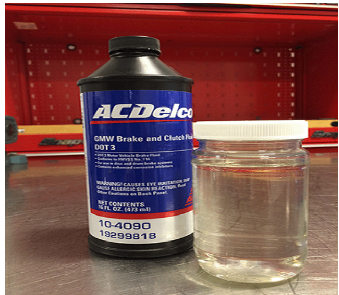
Diesel Exhaust Fluid (DEF) mixed with Brake Fluid.
