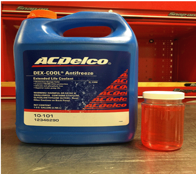
Diesel Exhaust Fluid (DEF) mixed with Dexcool.
