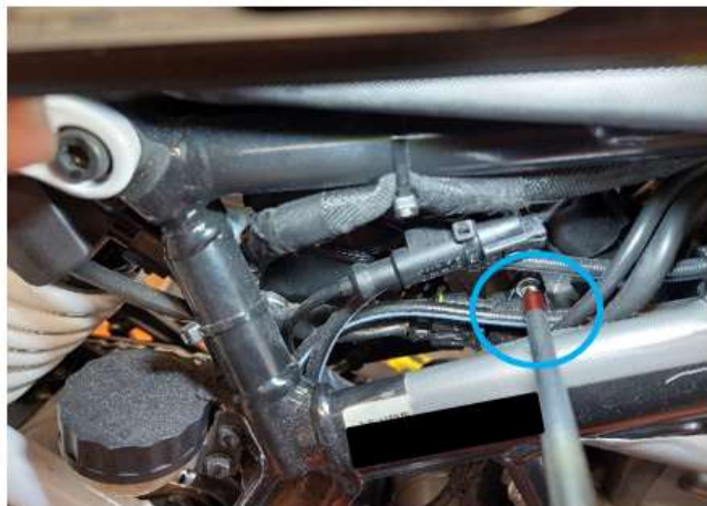
Fig. 4 – Removing the TPS screw connection
