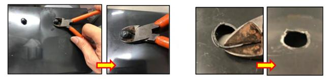
**CAUTION:** Be sure the protrusions are trimmed flush. The remaining protrusion height MUST be less than 2mm to provide proper fitment.
