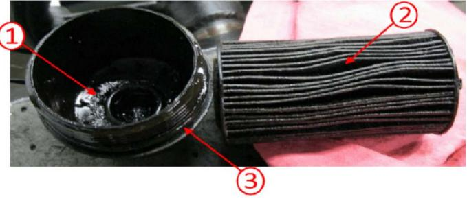
**Note:** Using care, some oil filters may need to be cut open in order to validate the condition of the filter.
