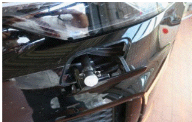
Figure 1. The headlamp washer nozzle jammed in the extended position.
