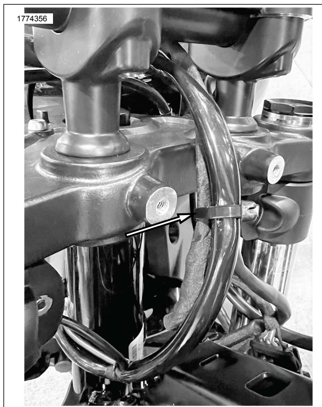
Figure 4. Harness Routing With Cable Strap
