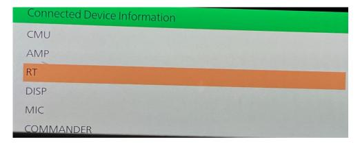
18. Check Device Name/Ver. Confirm that target software has been installed. For the target software, refer the table in the page 2.
