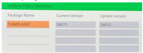
**NOTE:** Please DO NOT switch ignition or ACC OFF and do not remove the USB memory until all update files have been installed.
