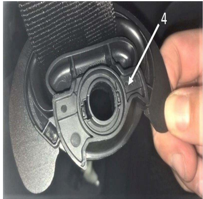
Figure 1. Seat belt deflector at height adjuster with B-Pillar trim removed.
