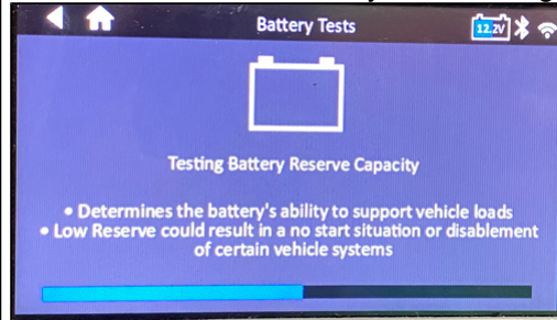
5. DCA-8000 will test battery before charging begins
