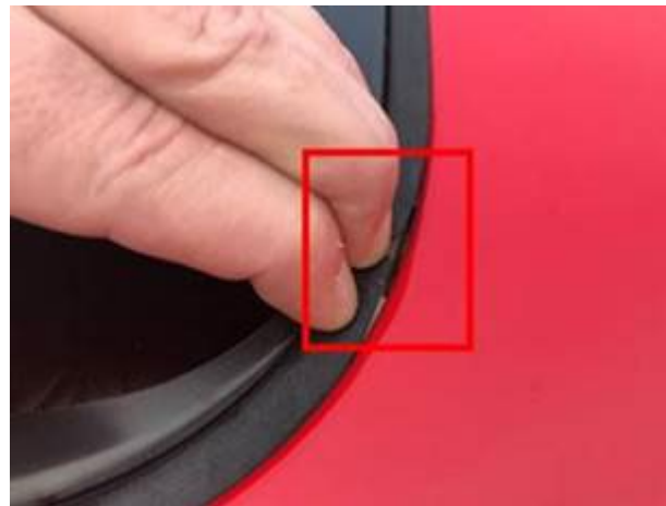
Figure 7. Adhesive band detachment.
