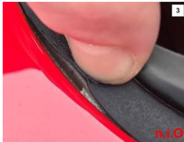
Figure 6. Seal adhesive band detachment revealed.
