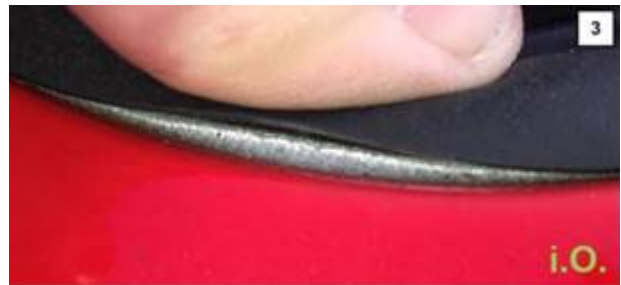
Figure 3. A properly adhered perimeter seal.
