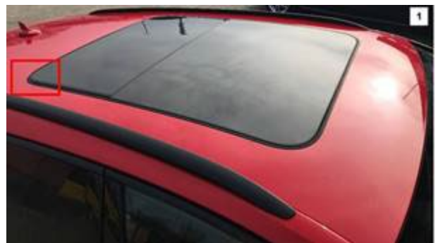
Figure 4. Begin inspection of the rear portion of the perimeter seal.
