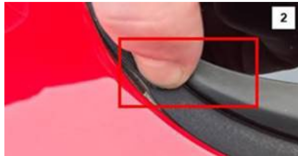
Figure 5. Clear evidence of adhesive detachment.
