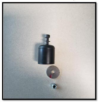
12. Install bumper assembly into the air box and install washer 20732084 and lock nut 990977.
