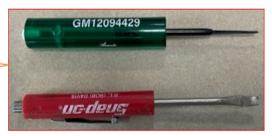
After lock has been removed you can use the terminal unlocking tool to unlock the wire terminal and slide the wire and terminal out the back side of the connector.
