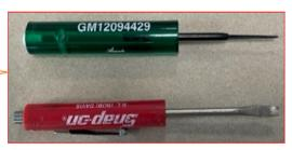
After lock has been removed you can use the terminal unlocking tool to unlock the wire terminal and slide the wire and terminal out the back side of the connector.
