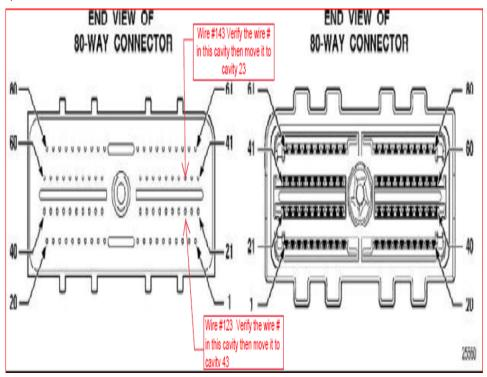
**AFL 80F Bolt-Assist Transmission Control Module** (TCM Connector)
