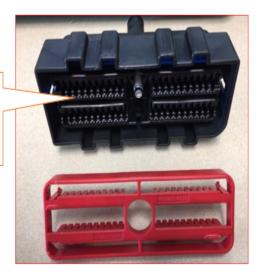
After you have swapped the wires in cavity 23 and 43, assemble the connector and plug it back in to the TECU and tighten the bolt. (DO NOT **OVER TORQUE)**
