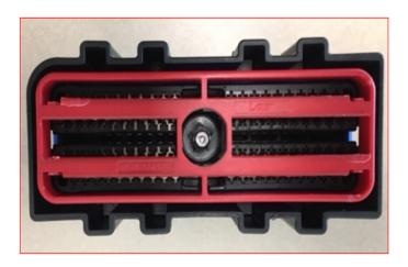
• After removing the 80-way connector, you will need to remove the red terminal lock terminal part #25193072 if needed
