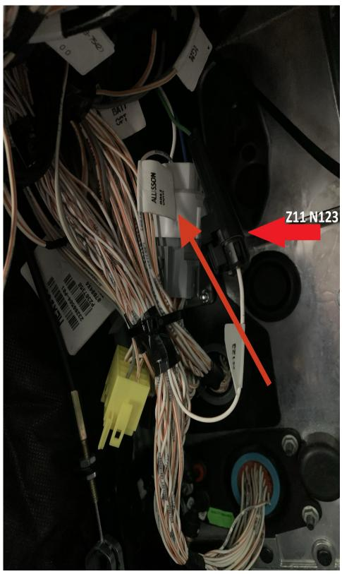
\*\*If either Connector Gray or Brown is fully Populated on the Body Builder Side look for the Round RP170A 31 Pin Connector located at the back of cab and remove the Body Builder Wire from Cavity 18 Live UI ive it to Cavity 19.
