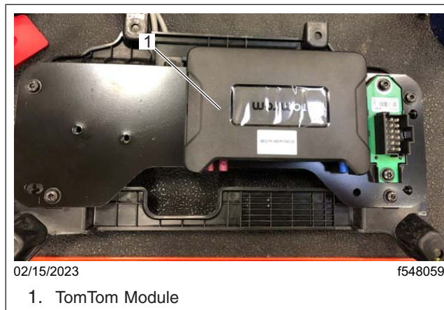
Fig. 11, TomTom Module Installation
