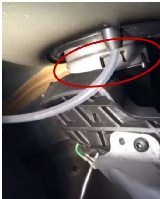
Figure 2. Check for smoke escaping around the filler neck.
