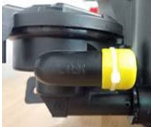
Figure 1. Block the filter port on the NVLD sensor.
