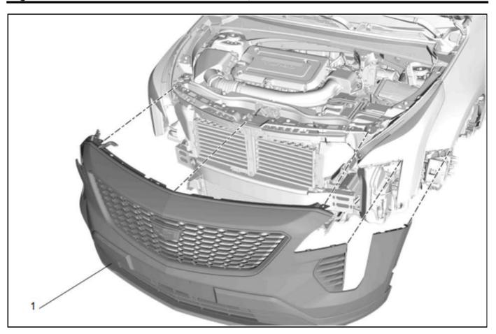
1. Remove the front fascia (1). Refer to *Front Bumper Fascia Removal and Installation* in SI.
