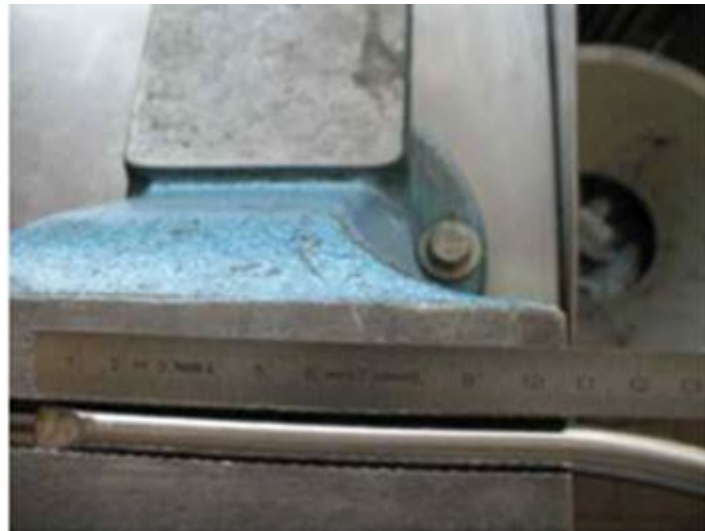
Figure 16. Rod inserted in a vice 11cm from the chisel end.
