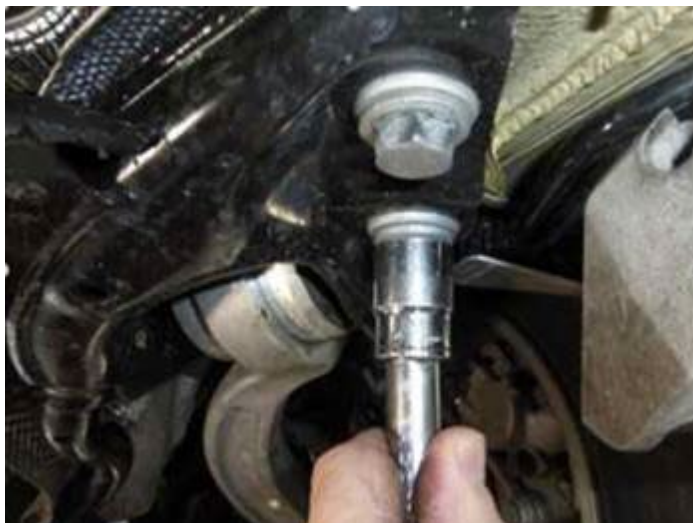
Figure 3. Loosening the front most subframe bolt.
