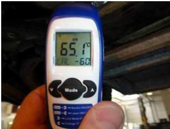
Figure 5. Surface temperature warmed to 65° C (149°F).
