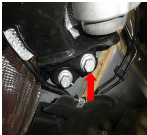
Figure 2. Front most bolt on subframe to be loosened.
