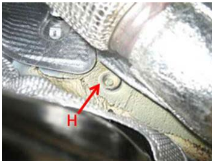
Figure 9. Remove grommet 'H'.
