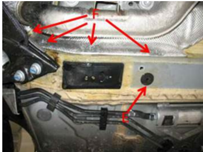
Figure 8. Gaining access to the longitudinal member.
