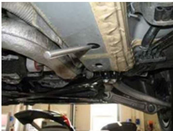
Figure 26. Steel rod driven forward at least 10mm.
