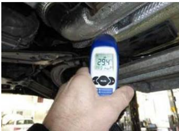
Figure 6. Surface temperature cooled to approximately 30° C (86°F).
