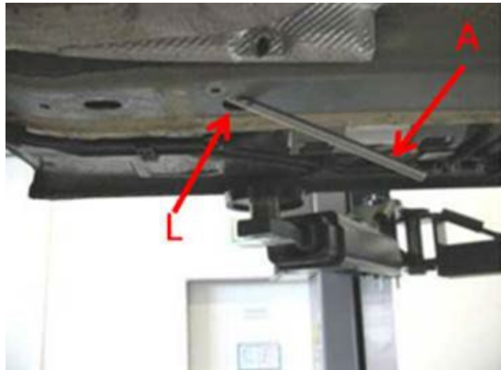
Figure 19. Insert the steel rod.
