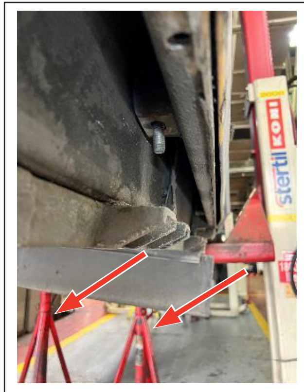
Figure 2 - View of Support system under the Tank and Cradle Assembly
