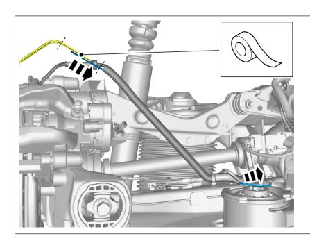
Use tape and attach the wire to the existing wiring harness.
