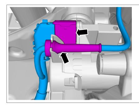
Disconnect the connector. Loosen the fastener.
