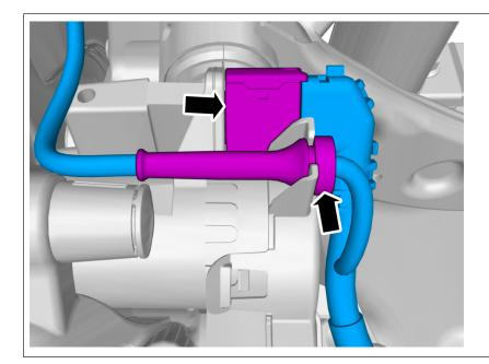
Disconnect the connector. Loosen the fastener.
