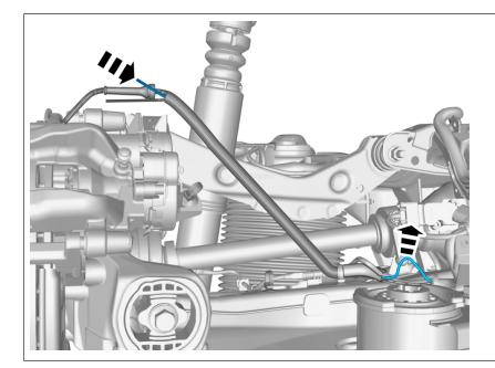
Pull the wiring through.
