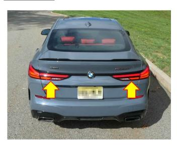
The trunklid-mounted inner taillamp turn indicators (arrows) do not function.
