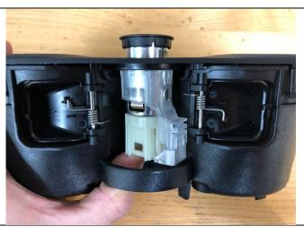
2. Push the original plug-in socket from the bottom up.
