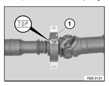
**NOTE:** The "TOP" designation on the center bearing points upwards towards the transmission tunnel.
