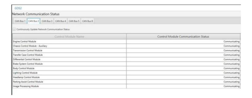
3) If after all modules are communicating and you continue to have issues or current DTC: U1962, then perform a Serial Data Authentication Configuration (SDAC), which is located on the SPS controller screen in the SPS, shown below. This will have to be completed so each module recognizes each other on their respective data buses.
