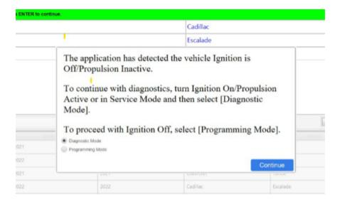
2) Next, use GDS2 Network Communication Status and check each CAN bus (1-8) to determine which modules are communicating and which modules are not communicating. This is similar to the Detected State feature of the Data Bus Diagnostic Tool (DBDT), but the DBDT will not work on these models. The GDS2 Network Communication Status can be found by following this GDS2 path: Vehicle Diagnosis/Vehicle Communication Diagnostics/Network Communication Status.
